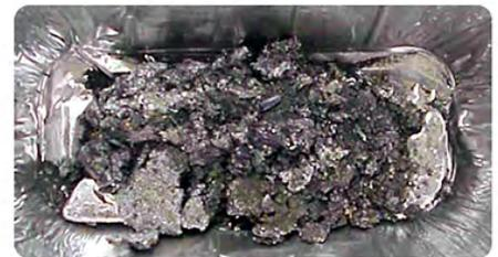
After just one hour in the AKILA unit, dross is converted to useable solder.
