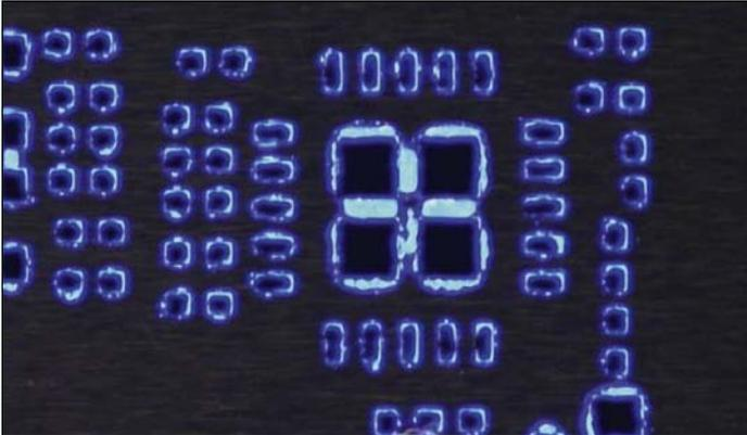
*Nanocoating helped to reduce the flux buildup on the bottom side of a stencil.*
