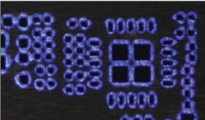
*For a stencil without nanocoating, the flux spread away from the apertures.*
